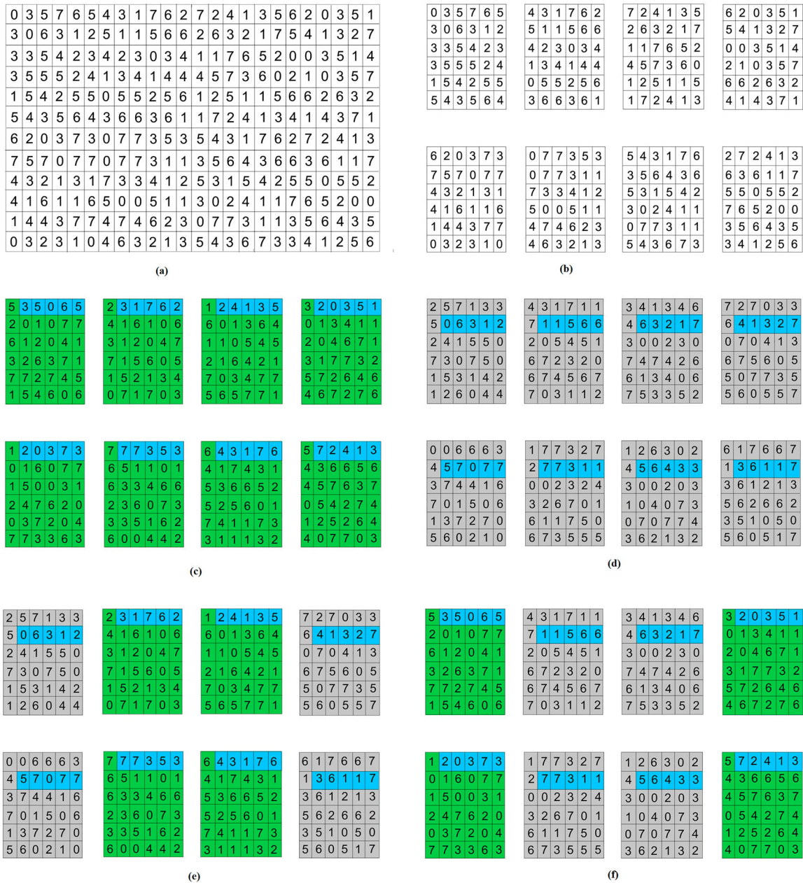
Figure 6. (a) Original image, (b) original image into eight equal parts, (c) first generation, (d) second generation, (e) third generation after double point crossover, (f) forth generation after double point crossover.
